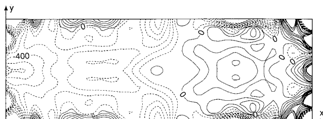
Fig. 4 Residual error in the transverse equilibrium equation E_3/L_{33\max} .
